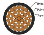
Extra fine bare copper conductor Polychloroprene rubber jacket Separator
